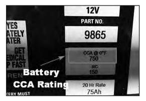
size can come in a range of CCA ratings. Using a battery with a higher CCA number is acceptable - even advantageous in some cases - and won't damage your car. A battery with more available cold cranking amps than the car manufacturer calls for just means that
