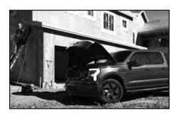
available Ford Intelligent Backup Power that can provide full-home power for up to three days on a fully charged battery, or as long as 10 days if rationing power. And you can turn your truck into a generator. The Pro Power Onboard feature offers an available 9.6 kW of max power provided through 11 outlets. No matter the job, the 9.6 kW version offers four 120V outlets in the front trunk, two in the cab, and four in the bed. The bed also features a 240V outlet for the tougher tasks at hand.
